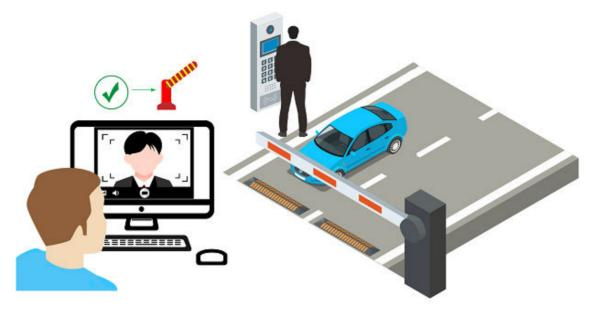
Figure 22-10 Opening Barrier by Video Intercom
