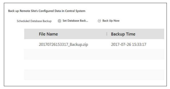
Figure 13-1 Back Up Remote Site Database in Central System
